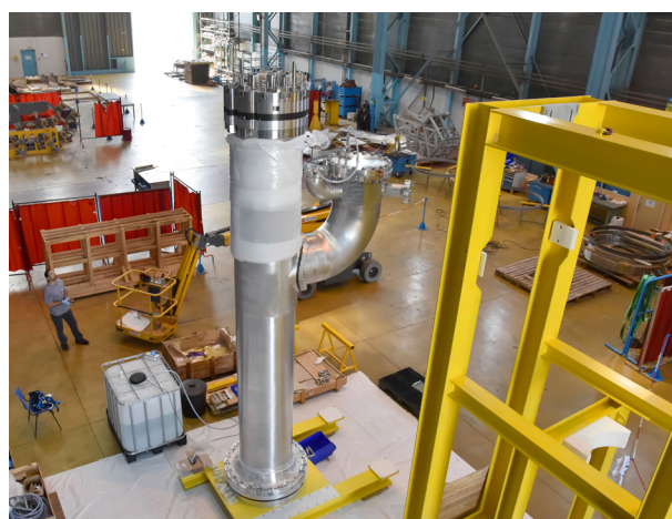
Core vessel and closure head for Jules Horowitz Reactor in France ©CEA
